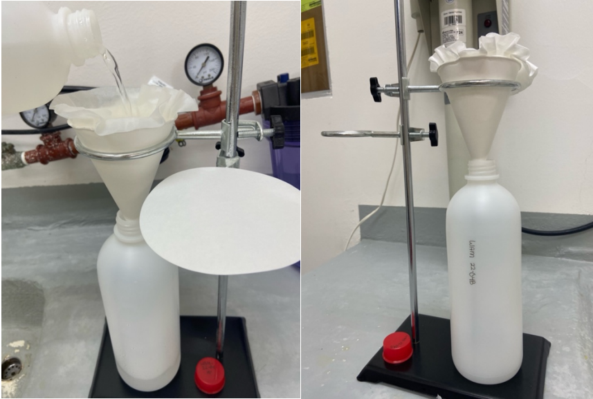
Image I. Gravity-drip apparatus with multi-sized filters (Newstar 110 mm coffee filter of Grade 103, 0.22-0.44 \mu\text{m} Sterivex filters, Newstar 100 mm coffee filter).
